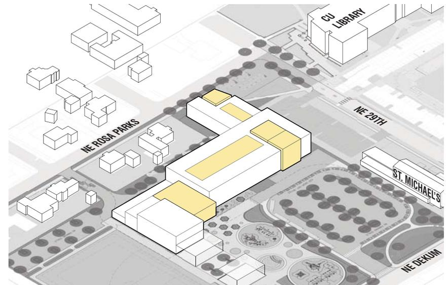
**INITIAL MASSING DIAGRAM.** This diagram shows basic relationships between the site and building. The collaborative core is shown in yellow.
